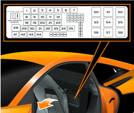
Main fuse box fuse specification chart
