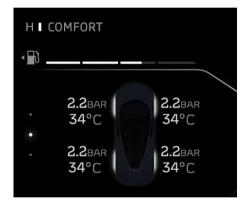
The display shows the pressures of each of the four tyres. If the tyre icon next to the pressure figure appears in white, no action is required. If it appears in red, inflate the associated tyre to the correct pressure as soon as possible.
