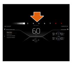
The tachometer display appears at the top of the Driver Display when in Non-Active or Comfort powertrain and handling modes. The red number on the display indicates the engine's maximum RPM.
