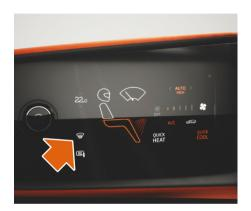
Touch the demist button to activate the screen demist function. The button will illuminate and an icon will be displayed at the top of the screen to indicate the function is active. The air conditioning switches on if previously off and the blower will operate at full speed with the air temperature set to 'HI'.
