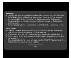
When the WCS initialises, either for the first time, or after a power outage event, it will calibrate the Base Pad. For this calibration to work, the Base Pad must be clear of any foreign objects. Because the calibration is essential for the correct operation of the WCS, it requires human interaction to confirm that the Base Pad is clear.
