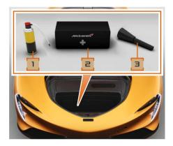
The emergency equipment is stored in a foam block, in a recess at the rear of the front luggage compartment:
