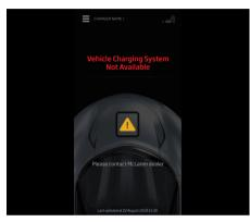
This error indicates a fault on the vehicle side of the charging system. The vehicle will not charge while the system is in this state.
