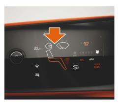
The air distribution can be set using the air distribution controls.
