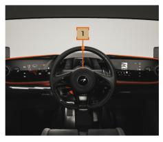
The driver's front air bag (1) deploys in front of the steering wheel.
