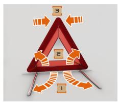
Fold the legs (1) sideways from the bottom. Pull side reflectors (2) upwards to form a triangle and lock them at the top using press-stud (3).
