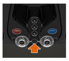
Pressing the ACTIVE button switches on the Active Dynamics Panel. This activates the Launch, ESC off, handling and powertrain controls. The ACTIVE button and handling and powertrain switches will illuminate.
