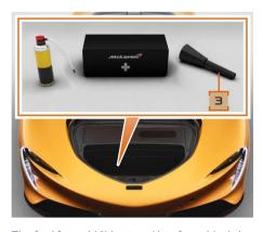
The fuel funnel (4) is stored in a foam block, in a recess at the rear of the front luggage compartment.
