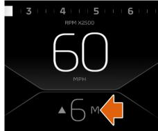
The gearbox mode indicator displays M and the currently selected gear. All forward gear changes are made by operating the gearshift paddles, see Gearshift paddles, page 2.16.
