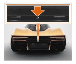
The rear view camera (RVC) is mounted in the centre of the rear bumper. The live video feed is displayed on the Driver Display when the function is active.
