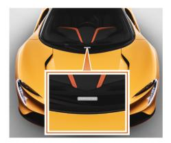
The vehicle identification number is located centrally, at the bottom of the windscreen.
