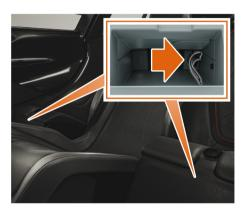
The internal door release strap is located inside the seat stowage compartment, see Seat stowage compartments, page 5.12.
