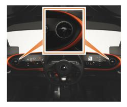
The dashboard air vents can be opened and closed by pushing the centre blade.
