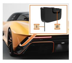
The key fob openeng tool (hex key) (1) is located inside the rear clam and can be accessed by reaching in, alongside the rear diffuser.
