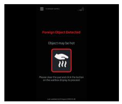
Foreign object on the Base Pad represents a potential hazard and will prevent charging from taking place. If the object is partially or wholly made of metal, heating of the object can occur. The WCS can detect if a foreign object is present on top of the Base Pad and will display the above screen.
