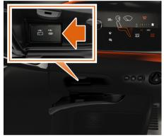
Two USB sockets are located inside each of the dashboard stowage compartments.
