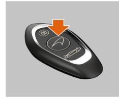
To unlock the vehicle, using the key fob, press the unlock button. The front, rear and side direction indicators flash twice and the anti-theft alarm system will be deactivated.
