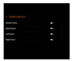
When Both doors is selected, both doors will unlock when the vehicle is unlocked using either the key fob or door button.
