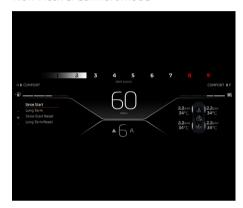
The display window provides the driver with visual access to the control settings and current performance values of the vehicle. The Driver Display, as indicated above, is displayed when the vehicle is in Non-Active/Comfort mode.
