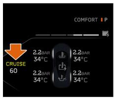
Accelerate to the desired speed and push the stalk up briefly, to activate cruise control. The set speed will appear on the Driver Display.
