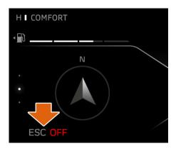
Confirmation of the electronic stability control mode selected is displayed. For more information on the different settings that are available, see Electronic stability control (ESC), page 2.30.
