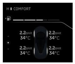
This shows the current temperature of each of the four tyres. If the tyre icons next to the temperatures appear in blue, the tyres have not yet warmed up to normal operating temperature. Do not exceed 75 mph (120 km/h) until the tyres have warmed up to normal operating temperature.
