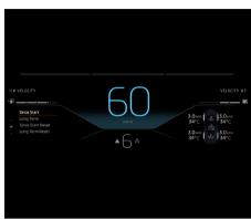
The display window provides the driver with visual access to the control settings and current performance values of the vehicle. The Driver Display, as indicated above, is displayed when the vehicle is in Velocity mode.
