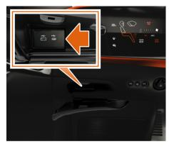
Open the dashboard stowage compartment and connect the device as required.
