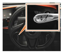
Navigation through the carousel menu structure is achieved using the control stalk mounted on the left of the steering column.
