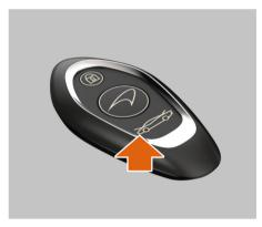
Press the front luggage compartment release button on the key fob, the front luggage compartment will fully unlock and open slightly.
