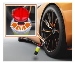
You can use the tyre sealant to seal small punctures, particularly those in the tyre's tread. The tyre sealant can be used at ambient temperatures down to -20°C (-4°F).
