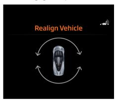
The vehicle may be skewed at an angle with respect to the Base Pad. While some coupling may be achieved in this position, adequate coupling may not occur. If this situation arises, the system will display the Realign Vehicle screen.
