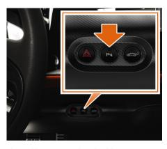
The parking sensors alert the driver to any obstructions while manoeuvring at low speeds. The system comprises four ultrasonic sensors in the front bumper, four ultrasonic sensors in the rear bumper and two sounders. Each sounder has a different pitch to indicate whether the obstruction is at the front or the rear of the vehicle.
