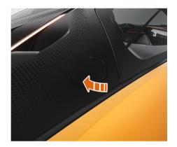
Press the rear edge of the service cover, the latch will release and the cover will open.
