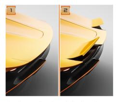
The ailerons adjust dynamically, dependent on the vehicle's requirements. This enhances vehicle stability with increased aerodynamic drag. The ailerons will operate at any vehicle speed.
