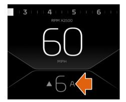
The gearbox mode indicator displays A. All gear changes occur automatically, but if a gearshift paddle is operated the gearbox will adopt a temporary manual mode. This mode will remain active for as long as the driver continues to make manual gear changes, each within an eight second period. The gearbox mode indicator displays A/M, see Gear position indicator, page 3.13.
