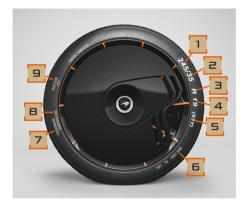
1. Width of tyre in millimetres.
