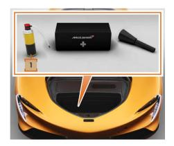
The tyre sealant (1) is stored in a foam block, in a recess at the rear of the front luggage compartment. Remove the first aid kit and release the two straps to remove the tyre sealant.
