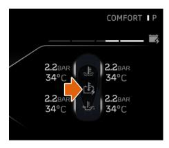
The High Voltage (HV) battery temperature icon is on the right-hand side of the Driver Display.
