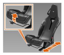
Lift the lever, move the seat to the desired position and release the lever to lock the seat.
