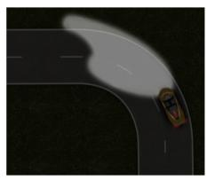
With the headlamps on, the Static Adaptive Headlamps adjust the beams when cornering, providing improved illumination in the direction of travel.
