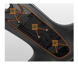
4. Remove the six nuts (2) from the underside of the engine cover.
