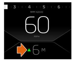
When in manual mode and driving more economically, the gear shift indicator (GSI) will illuminate when an upshift would maintain optimum economy. The GSI will not illuminate if the requested acceleration or deceleration cannot be met with a higher gear. See Economical driving, page 2.10.
