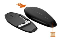
Using the hex key provided, remove the screw 1, then lift the back cover away from the key fob.
