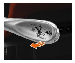
Pull the cruise control stalk briefly towards you. Cruise control will adjust the vehicle's speed to the last speed stored.
