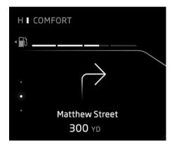
The current navigation turn-by-turn guidance will be displayed on the Driver Display if route guidance has been started using the McLaren Infotainment System (MIS).
