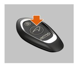
If either the doors or the luggage compartments are left open, or the key fob is still inside the vehicle, the horn will sound indicating mislock when an attempt to lock the vehicle is made.
