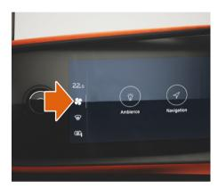
The climate control system is operated using the left-hand McLaren Infotainment System (MIS) screen. Touch the climate control icon to expand the application and access all controls.
