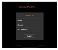
Once your phone has paired and connected to the MIS, select whether to connect as Phone 1 or Phone 2. Select No connection if the Bluetooth® device is to be used for audio streaming only.
