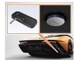
6. The mechanical lock is located in the rear diffuser, on the right-hand side.
