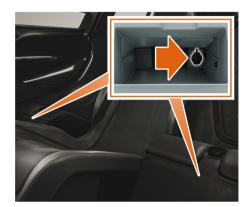
A 12V accessory socket is located inside each of the passenger seat stowage compartments and each have a maximum load rating of 15 Amps.
