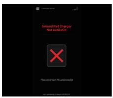
This error indicates a fault in the Base Pad charger portion of the charging system. The vehicle will not charge while the system is in this state.
