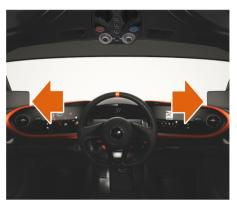
The live video feed is displayed on the two outer screens when the function is active.
