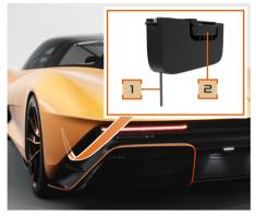
The manual door release key holder (2) is located inside the rear clam and can be accessed by reaching in, alongside the rear diffuser.
