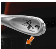
Accelerate or decelerate to the maximum permitted speed and push the stalk down briefly, to activate Active Speed Limiter (ASL).
