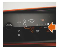
Select air recirculation when unpleasant smells or fumes are entering the vehicle. Air from outside the vehicle is now prevented from entering the cabin.
