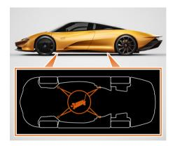
Refer to the illustration, and labels on the vehicle, for correct lifting locations.
