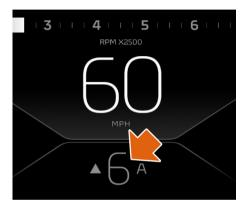
The gear indicator shows the current gear position selected: Neutral, Gear 1-7, or Reverse. The indicator will also show A or M depending on whether automatic or manual mode is selected.
