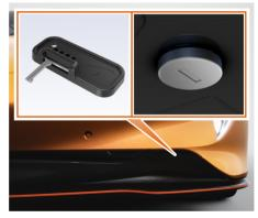
The mechanical lock is located in the front left-hand air duct.
