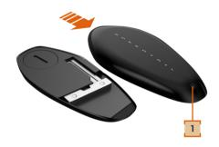
2. Release and remove the mechanical key from the key fob.
