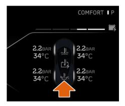
The oil temperature icon is on the right-hand side of the Driver Display.
