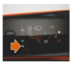
The CMS cameras can be heated in order to remove frost and condensation from the lens, see Heated Camera Monitor System (CMS) lenses, page 5.09.
