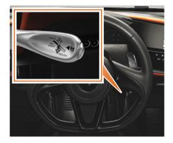
All cruise control functions are operated by the cruise control stalk, positioned on the right of the steering column.
