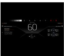
The display window provides the driver with visual access to the control settings and current performance values of the vehicle. The Driver Display, as indicated above, is displayed when the vehicle is in Sport mode.
