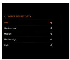
Select the sensitivity level to suit your preference for wiper operation. This setting will apply for the rain sensor sensitivity level only and will not affect the intermittent wipe time delay.
