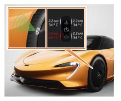
The tyre pressure monitoring system warns you when the pressure drops or the temperature increases above an acceptable level in one or more of the tyres.
