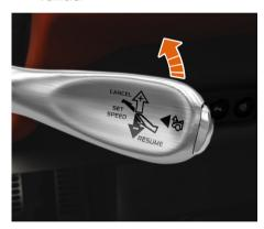
Before vehicle lift can be activated, the engine must be running. To raise the vehicle, activate the vehicle lift menu (see Vehicle lift operation, page 1.36) and then move the control stalk upwards.
