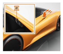
Firmly press and hold the rear button (2), located within the side duct, for two seconds to close the door. Once the door has started to close, the button can be released and the door will continue to close fully.
