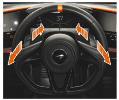
To upshift, pull the right-hand paddle towards you. To downshift pull the left-hand paddle towards you. The current gear position appears on the gear position display, see Gear position indicator, page 3,13.
