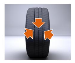
When the tread is worn to 1.6 mm, the wear indicators appear on the surface of the tread pattern, producing a continuous band of rubber across the width of the tyre. Tyres must be replaced as soon as the wear indicator becomes visible, or sooner if legislation dictates replacement at a greater tread depth.
