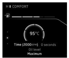
Displays a gauge showing the level of oil, together with the oil temperature.
