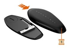
Using the hex key provided, remove the screw 1, then lift the back cover away from the key fob.
