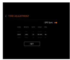
GPS sync automatically adjusts the time using the GPS signal. Touch GPS Sync to toggle the function On or Off.
