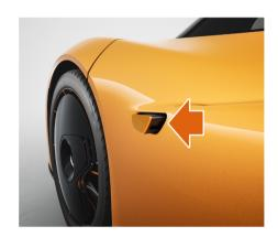
The Camera Monitor System (CMS) replaces the conventional exterior mirrors with a camera mounted on each side of the vehicle, just behind the front wheels. The cameras are automatically deployed when the vehicle is unlocked and retract again when it is locked. The feature can be disabled and the cameras permanently deployed, see Automatic Folding, page 4.12.
