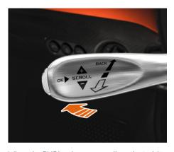
When the RVC has been manually activated, it can be deactivated by pushing the control stalk away from you.
