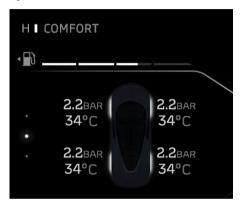
This shows the pressures and temperatures of each of the 4 tyres. If the tyre icon next to the pressure or temperature figures appear in white, no action is required. If they appear in amber or red, have the tyres inspected and pressures rectified as soon as possible.
