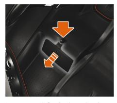
A compartment is fitted underneath each seat for storing small items.
