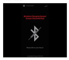
This error indicates that the tablet has stopped receiving messages from the WCS, because the Bluetooth connection between the Wall Box and the tablet has been lost. This error is often transient and it may disappear after a few minutes, without any user intervention.
