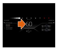
The speedometer is situated centrally on the Driver Display when in Non-Active or Comfort powertrain and handling modes.
