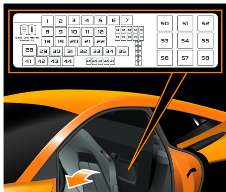
Main fuse box fuse specification chart
