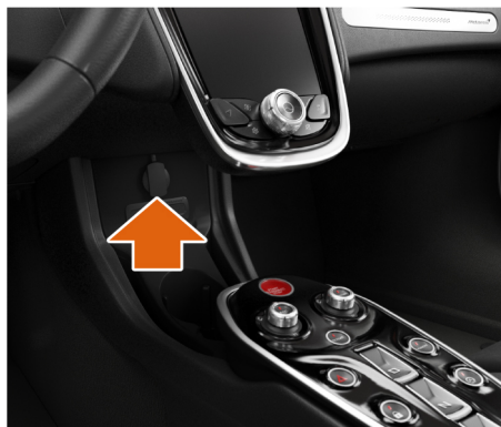
Interior accessory 12 V socket
