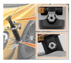
The rebound adjuster is located at the base of the damper body, rebound adjustment has 35 different positions. The adjustment wheel should be rotated clockwise to stiffen and counter clockwise to soften.
