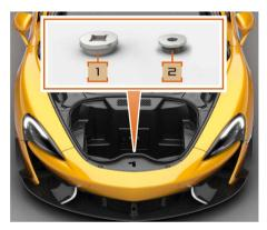
The wheel nut centre locking ring removal (2) and nut torque (1) tools are located in the front luggage compartment.
