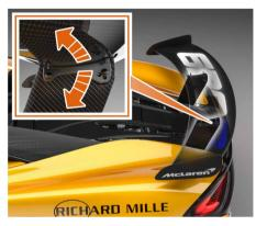
Rear wing adjustment 9 Nm (7 lb.ft) bolt torque figure
