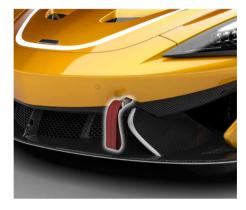
Your McLaren is equipped with a front tow strap, for use on track.
