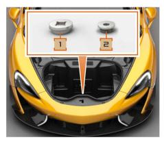
The wheel nut center locking ring removal (2) and nut torque (1) tools are located in the front luggage compartment.
