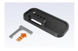
3. Insert the mechanical key into the manual door release key holder.
