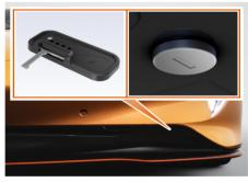
The mechanical lock is located in the front left-hand air duct
