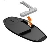
2. Release and remove the mechanical key from the key fob.
