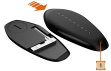
Using the hex key provided, remove the screw 1, then lift the back cover away from the key fob.
